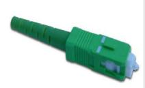
Description: The SC connector holds a single fiber in astandard-sized (2.5 mm) ceramic ferrule. The connector body has a square front profile, and ismade of moulded plastic. Clips on either side of the body and the connector key allow for easypush-in connections. This push-pull latchingmechanism makes the SC connector preferred inhigh-density interconnect
